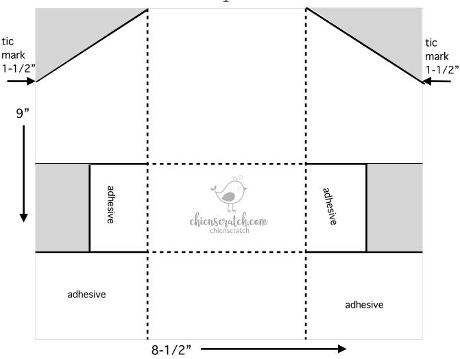
Score on Dotted Lines - Cut on Solid Lines - Remove Shaded
